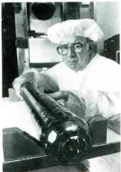
WESTINGHOUSE TECHNICIAN Don Nebel holds a single-crystal boule of silicon, believed to be the purest and largest ever produced.
